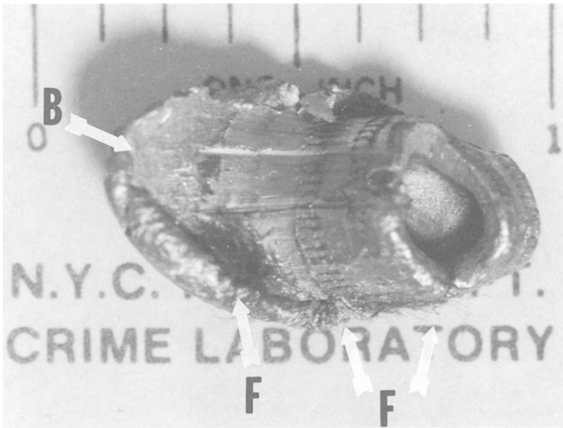
FIG. 3—A spent deformed bullet (B) with several tufts of fibers (F). The scale equals 1 in. (2.54 cm).
